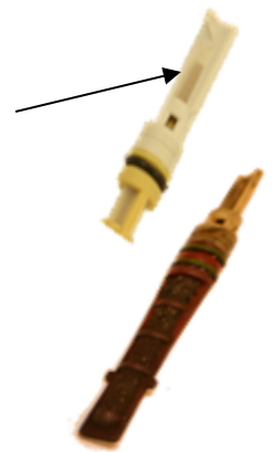
Figure 1.1 • The color of the orifice tube identifies the diameter size.
